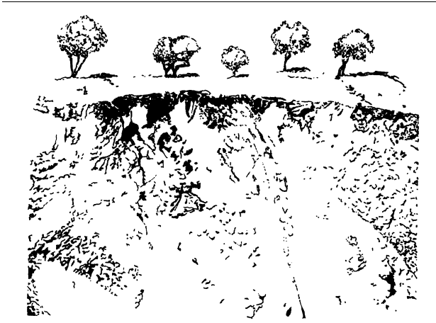
Figure 4-1: Residual soil forming from the in-place weathering of igneous rock
