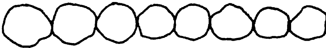
Figure 4-7: Uniformly graded soil
