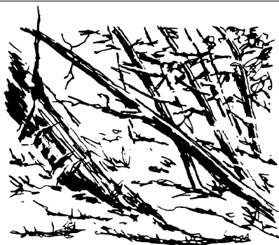
Figure 10-8: Backward rotation of a slump block
